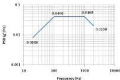
Figure 2. Random Vibration on Mounted Airborne Store
