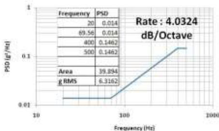
Figure 1. Random Vibration for a Typical Airborne Missile
